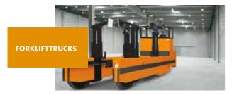
Heavy load 4-way sideloader in the glassindustry with wheels ø 1100 mm.
